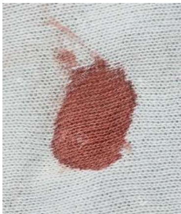
Fig 4: A 23 mm diameter bloodstain produced on cotton knit from a dropping height of 5 cm (0.091 mL)
