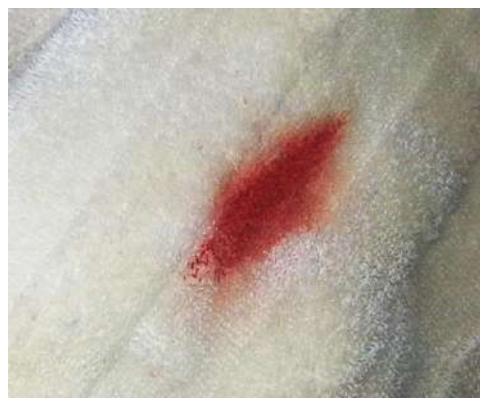
Fig 7: A 15.7 mm diameter bloodstain produced on heavy cotton from a dropping height of 180 cm (0.091 mL at 50°)
